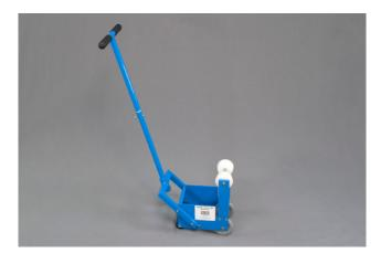
3. Remove the white plastic core roll core pieces by loosening cross bolt and pulling the pin as shown in the picture. Insert white plastic pieces into the core of the APEEL cover tape roll. Position the roll of cover tape in the applicator, reinsert pin through the white plastic pieces and tighten bolt to hold in place.
