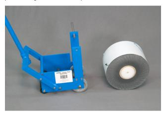
4. Using hands, pull cover tape down through applicator with the sticky side down. Pull tape beneath the gray roller and position under the 6 segmented pressure wheels as shown and begin applying.
