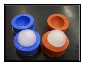
The ice spheres are initially weighed to 0.01 gram and then placed in the barrel, similar to a lead shot for a muzzle loader. As the ice sphere is pneumatically launched towards the target, the velocity is measured with a ballistics timer. The kinetic energy, or "impact energy", is then calculated for each hail shot. The minimum kinetic energies listed by the NBS are maintained within a tolerance of plus zero plus ten percent.
