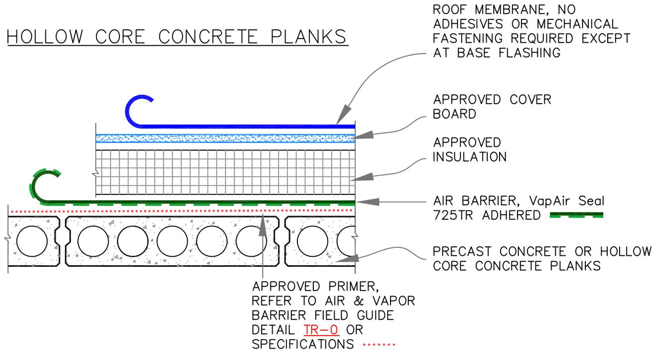
HOLLOW CORE CONCRETE PLANKS WITH TOPPING
