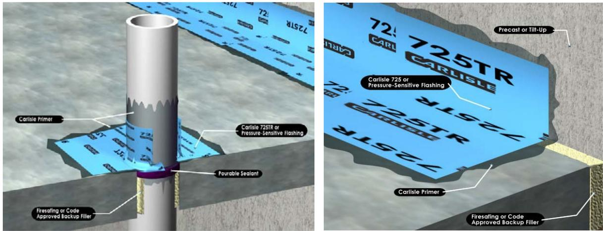
Gaps must be filled with firesafing or building code approved backup filler. Carlisle's VapAir Seal 725 TR or Pressure-Sensitive Flashing can be used as shown in illustrations after priming the substrate. For VapAir Seal 725 TR, use as a substrate primer Carlisle's CAV-GRIP, CAV-GRIP III, CCW 702, CCW 702LV or CCW 702 WB and for the Sure-Seal® Pressure-Sensitive Flashing, use Carlisle's EPDM Primer.
