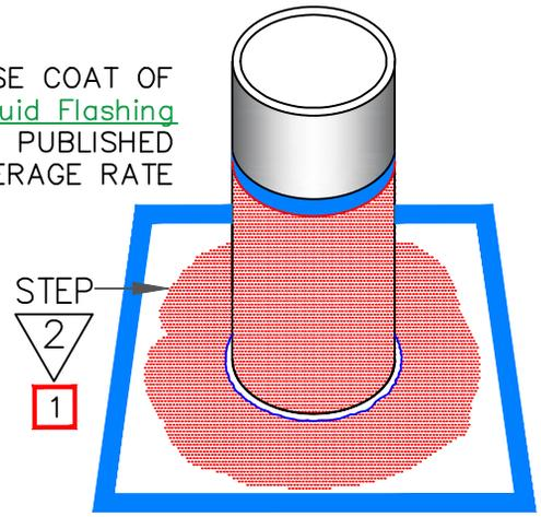
APPLY BASE COAT OF LIQUISEAL Liquid Flashing Resin ON HORIZONTAL SURFACES. IMMEDIATELY PRESS FLEECE INTO RESIN AND OVERLAP LIQUISEAL Flashing Fleece, MIN. 2" (51mm)
