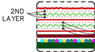
FIRST LAYER OF FLEECE 6.75" (171.5mm) EQUALLY EXTENDING BEYOND SEAM EDGES AS DEPICTED. SEE INSET ABOVE FOR DETAILED INSTALLATION.
