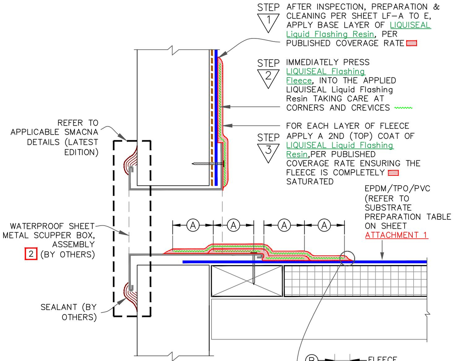
STEP 1 AFTER INSPECTION, PREPARATION & CLEANING PER SHEET LF-A TO E, APPLY BASE LAYER OF **LIQUISEAL Liquid Flashing Resin**, PER PUBLISHED COVERAGE RATE
