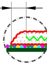
APPLY A TOP COAT OF LIQUISEAL Liquid Flashing Resin, ENSURING THE FLEECE IS COMPLETELY SATURATED PER PUBLISHED COVERAGE RATE AND APPLY 1/4" - 1/2" (7mm - 13mm) BEYOND THE FLEECE EDGES
