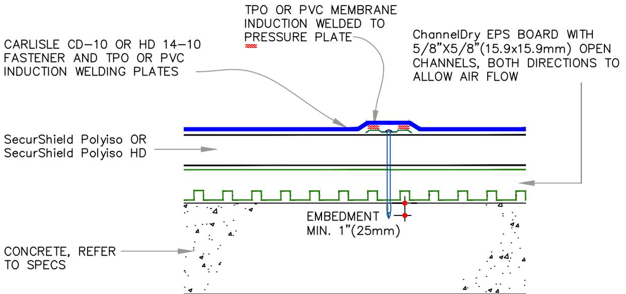
**D** TPO OR PVC INDUCTION WELDED ASSEMBLY
