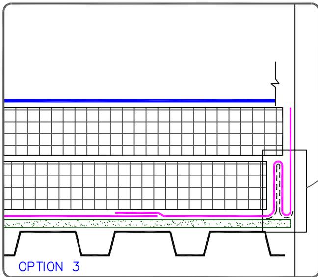
CONTINUOUS STRIPPING OF SELF-ADHERING VAPOR RETARDER 725TR FULLY ADHERED TO WALL AND SUBSTRATE WITH DOUBLE FOLD CREASES MIN. 2" (51mm) HIGH, SET VERTICALLY UP AGAINST THE WALL. DO NOT ADHERE THE FOLDS TOGETHER
