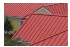
Our CM 150SS roof system will lend striking dimension to any architectural design. This versatile  $1-\frac{1}{2}$ " mechanically seamed panel can be curved to a wide range of radiuses and applications – from barrel roofs to conical shapes and more. Concealed fasteners and a floating clip system reduce the effect of thermal stresses on the panels, helping to maintain a beautifully smooth, uniform appearance despite fluctuations in temperature.
